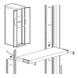
**Recessed horizontal mounting.** You can mount the Rack PDU in a recessed configuration by attaching the brackets in alternate positions on the PDU, as shown below.
